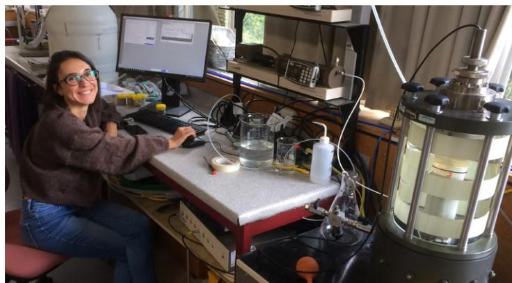
*Jordanka conducting triaxial tests. The triaxial apparatus (on the right) puts controlled stress on our tephra samples so we can study their response. This helps us relate the liquefaction within the tephra to past earthquakes.*
